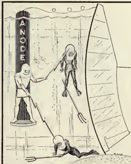
A SACRIFICIAL ANODE takes the corrosive action upon itself, turning the radial gate into a cathode. The protective anode is connected by a wire to the submerged metal structure. Illustrations by Marie L. Lang, Design and Construction Division, Denver, Colo.
